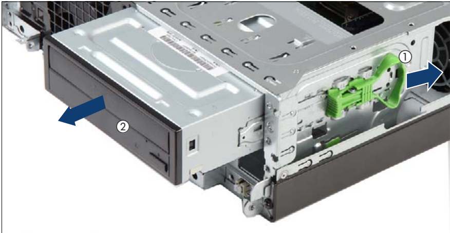
Figure 57: Removing HH ODD
